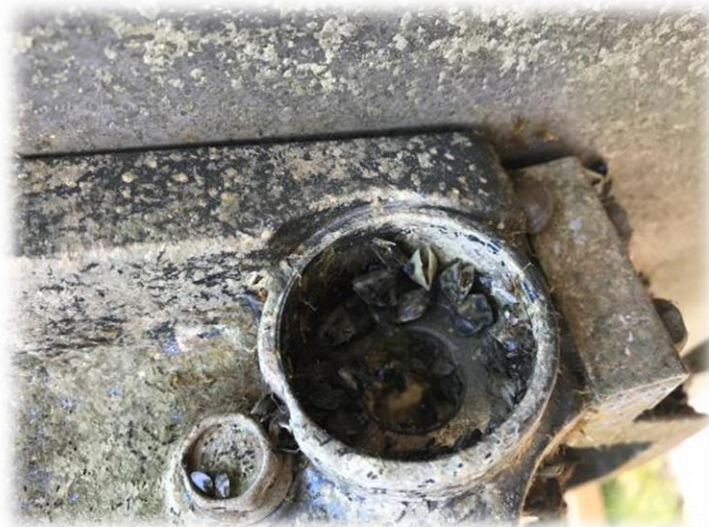
Zebra mussels crusted underneath a pontoon boat
